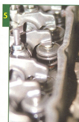
5 You can see when the valve is fully open. Pictured is valve five
